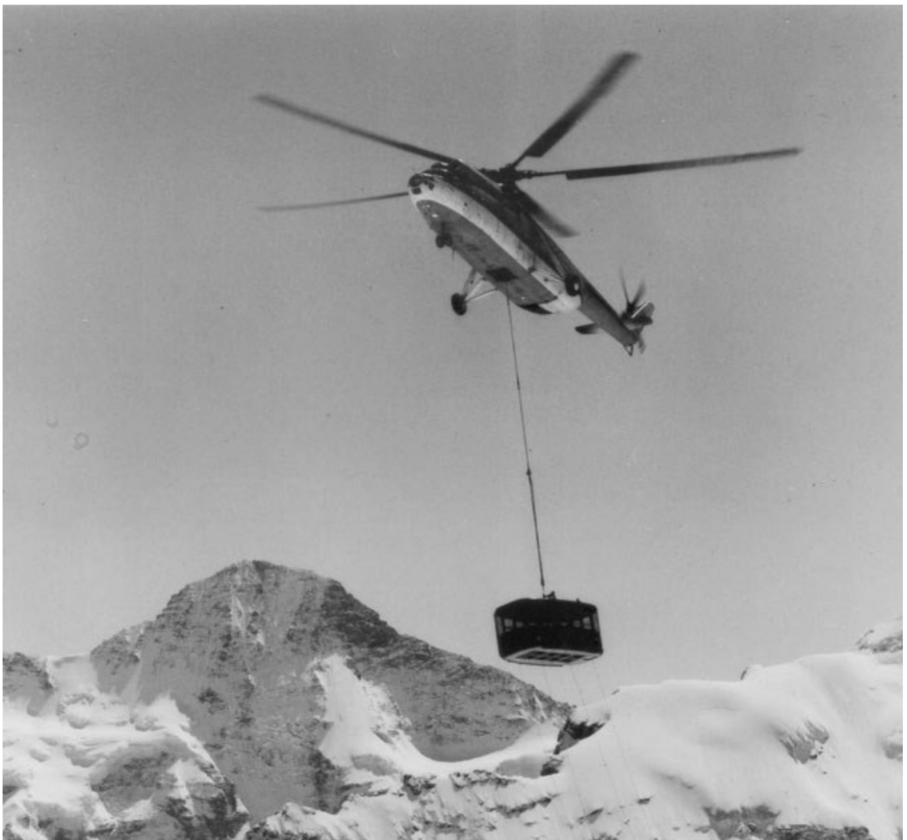
Stechelberg/BE, April 1966 - The Mil Mi-6 CCCP-06174 photographed before the transportation of one of the two new Schilthorn's cable car cabins (W. Studer - HAB)
